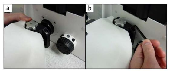
Figure 5.4.2(a)Engaging Clarity onto the microscope adapter, (b) locking the microscope clamp.
