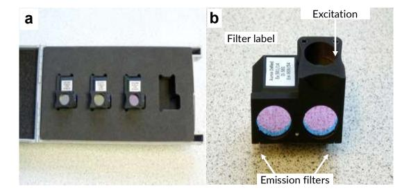
Figure 5.2.1(a) Filter cube case with three filter cubes, (b) Close-up photograph of a filter cube showing their positions and labelling.
