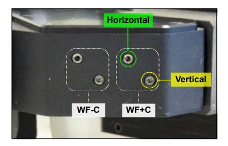
Figure 5.4.9(b)Camera alignment control screws
