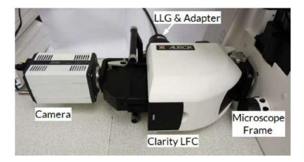
Figure 5.1 Fully assembled Clarity system with Liquid Light Guide and collimating adapter, scientific camera and microscope frame.
