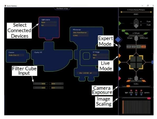
Figure 5.4.8 Visionary Hardware Set up Screen
