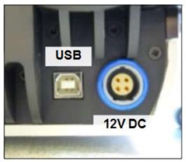
Figure 5.4.3 Clarity power and USB connections.
